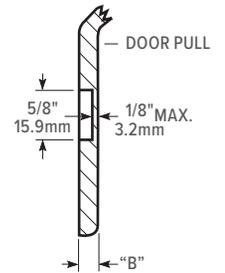
IF "B" dimensions exceeds 1/4" c'bore back side as shown to facilitate assembly. c'bore requirement does not affect spindle length determinaion.
