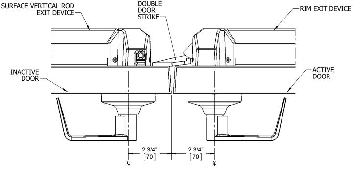
THE 4911 DOUBLE DOOR STRIKE IS FOR A PAIR OF DOORS WITHOUT A MULLION AND WITH A RIM EXIT DEVICE AND A VERTICAL ROD EXIT DEVICE. THESE DEVICES ARE MOUNTED WITH A 2-3/4" BACKSET. THE STRIKE IS TO BE MOUNTED ON THE INACTIVE DOOR, AND TO WORK IN CONJUCTION WITH THE ACTIVE DOOR.
