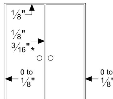
\* Allow extra clearance as required per astragal manufacturer. Certain door and frame conditions may require an extra 1/32"-1/16" clearance. Excessive clearance on fire rated assemblies may violate the requirements of NFPA 80.
