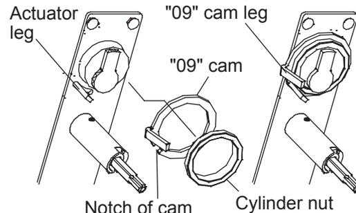
Due to individual cam configurations and cylinder lengths, the leg of the "09" cam may have to be bent slightly to function properly. 95054195 "09" Pack
