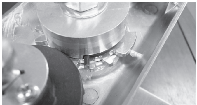
SPRING ORIENTATION FOR RIGHT HAND REVERSE OPERATION
