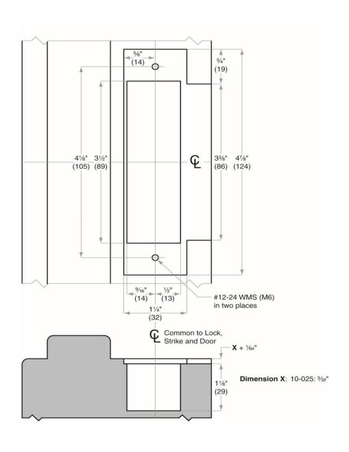
Note: Dimensions shown in brackets [] are in millimeters.
