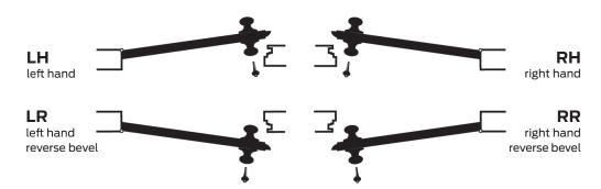
The hand is determined by the direction the door swings when viewed from the exterior or corridor side of the door.
