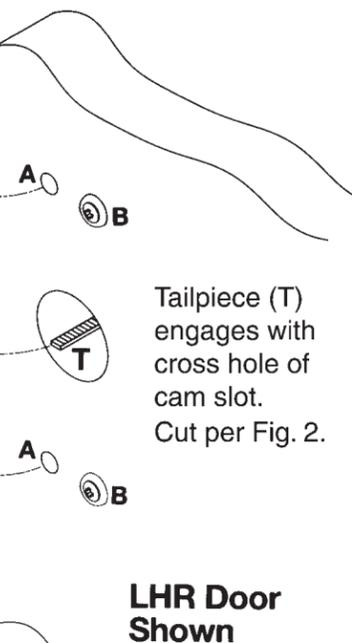
(2) Screws and washers bolt trim to door using holes "B".
