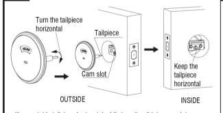
Keep outside tailpiece horizontal while inserting it into cam slot.
