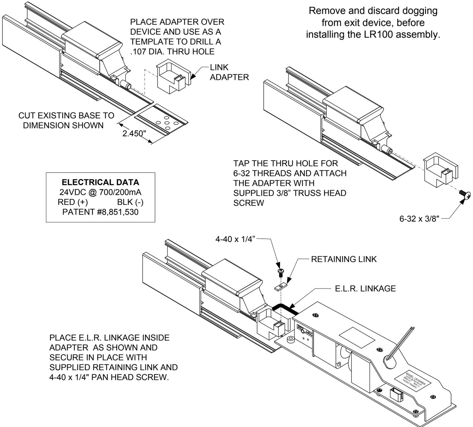
Remove and discard dogging from exit device, before installing the LR100 assembly.
