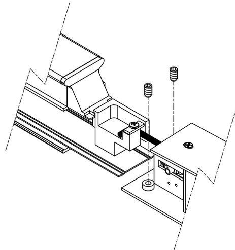
**Retrofit Installation Note:** 42" or 48" exit devices that have been modified to fit a 36" or smaller opening, may not have the required space to fit the standard E. L. R. assembly. Always verify the distance from the end of the touchpad to the end rail, and if necessary, consult with the factory for appropriate selection.
