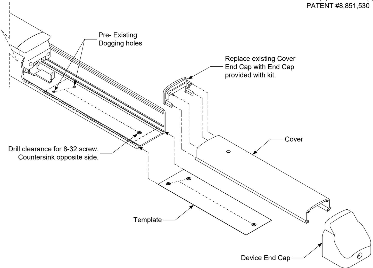
Slide the ELR assembly into the rail extrusion over the Dogging Arm within the device. Loosen the Catch Screw if required to allow for the ELR to be inserted over Dogging Arm. Fasten the ELR assembly to the rail extrusion of device as illustrated below using the provided mounting screws from ELR kit.
