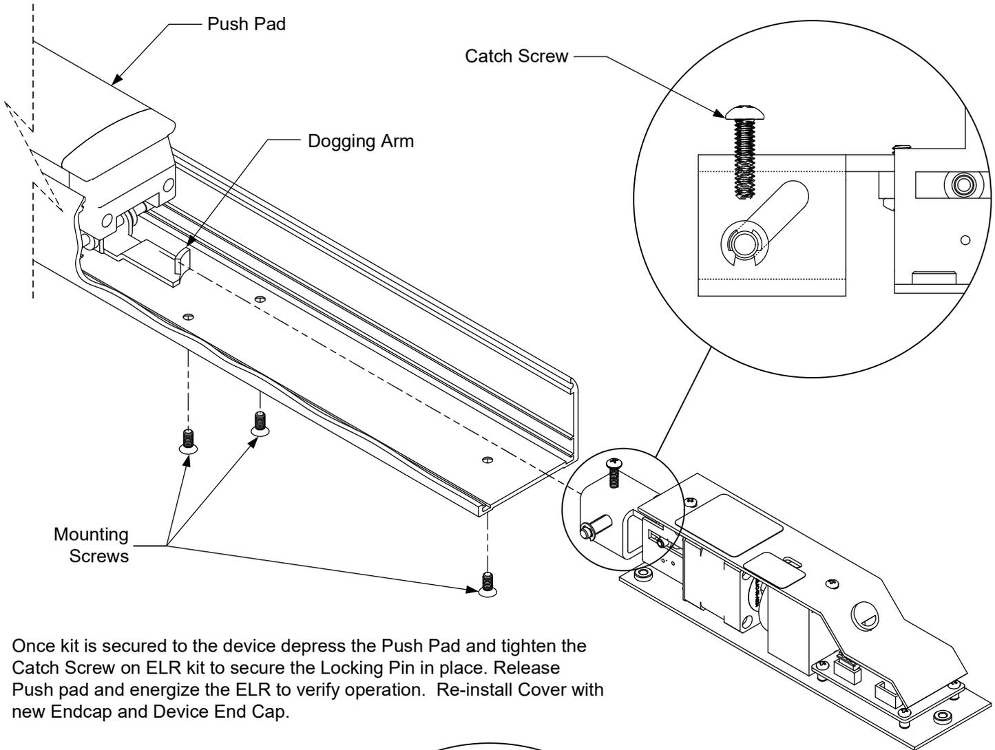
Once kit is secured to the device depress the Push Pad and tighten the Catch Screw on ELR kit to secure the Locking Pin in place. Release Push pad and energize the ELR to verify operation. Re-install Cover with new Endcap and Device End Cap.
