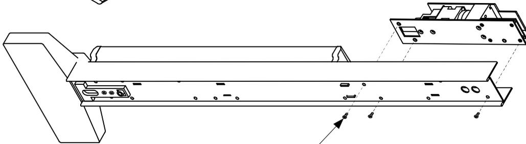
Replace Housing Cover, Cover with Plug, End Cap and the End Cap Cover.
