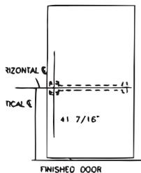
IDENTIFY TYPE OF INSTALLATION TO DETERMINE LOCATION OF VERTICAL &
