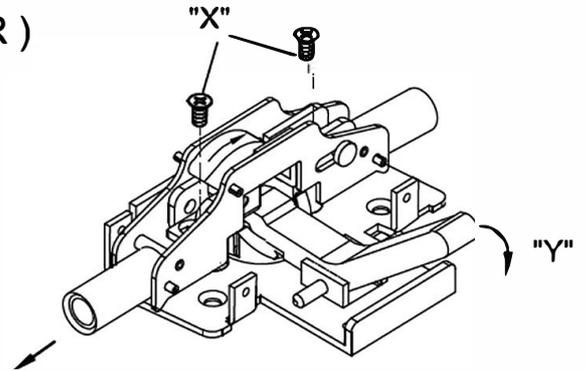
Fasten "X" at above screw hole position. Press Lift Arm "Y" to ensure the processing direction is reversed.
