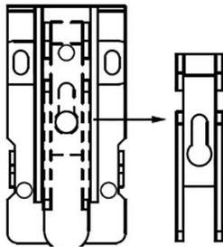
(2) Follow TEMPLATE to install top latch with two screws (B2) then screw (B1).
