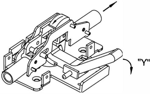
Press Lift Arm "Y" and ensure the direction before changing.
