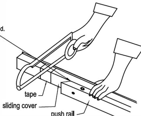
NOTE : the minimum length of the sliding cover must be 1" (25.4mm) or longer than length "C".
