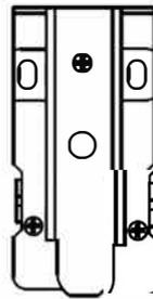
(3) Put the Linkage Into the top latch case.
