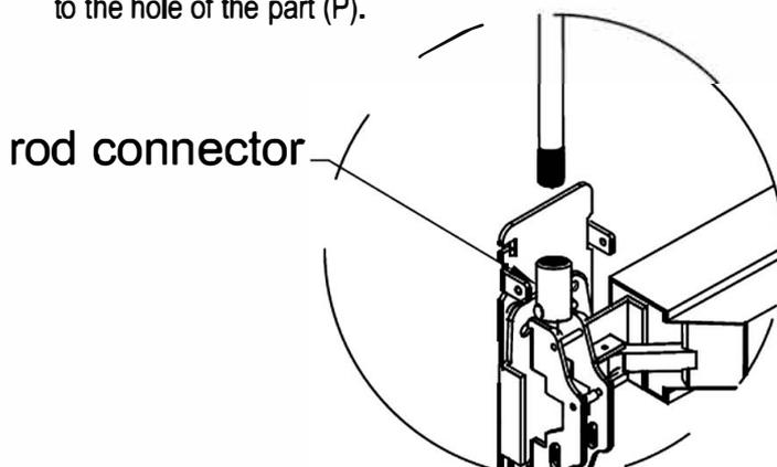
※ If top rod had been cut to fit door height, please drill hole for pin loading.
