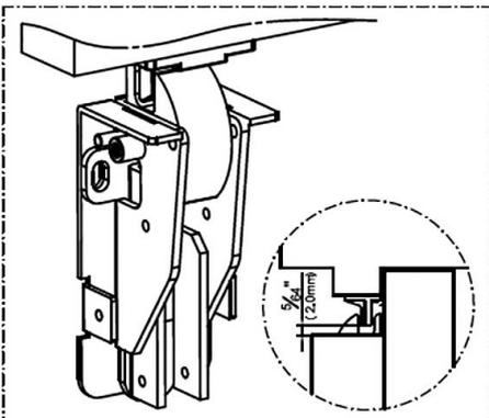
(5) Insert the Pin through the latch case and Top Latch.
