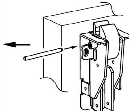
(4) Put the Top Latch into the top latch case.
