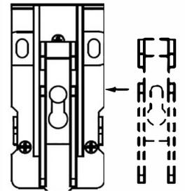
(6) Follow TEMPLATE to install top strike. Adjust the Proper gap between top latch and strike which is about  $\frac{5}{64}$ " (2.0mm).
