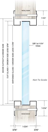
Designed for Use on 1¾" Thick Doors Manufactured Within Door Industry Tolerance of +/- ¼e".
