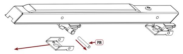
**3. Install Point of Front Activating bracket i**nto opening of motor's lifting bracket, resting on top of the nylon roller. Once in place, re-install the FRONT activating bracket PIN.
