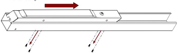
Locate and Remove the FRONT activating bracket by pushing out the PIN.
