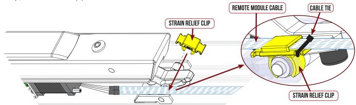
**7.** Test function and adjust PTS location, if needed (see page 4). Once complete, adhere cable tie mount, install cable tie, and adhere the MM5 assembly to the housing. Install filler plate and device end cap to finish the installation.
