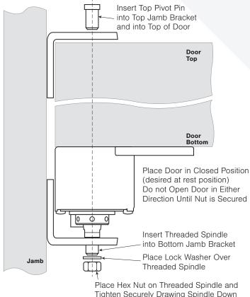
Tighten Securely Drawing Spindle Down into the Bottom Jamb Bracket
