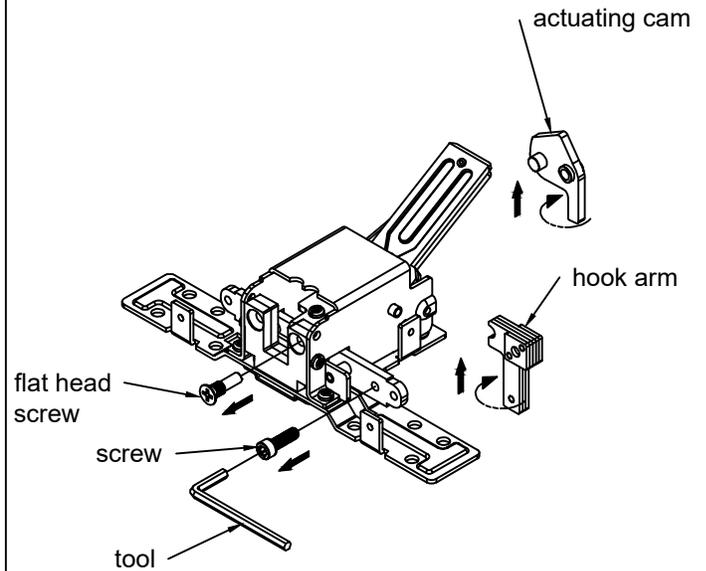
3-1. Reassemble actuating cam & hook cam at opposite side, as shown.
