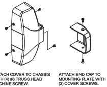
ATTACH COVER TO CHASSIS WITH (4) #8 TRUSS HEAD MACHINE SCREW.
