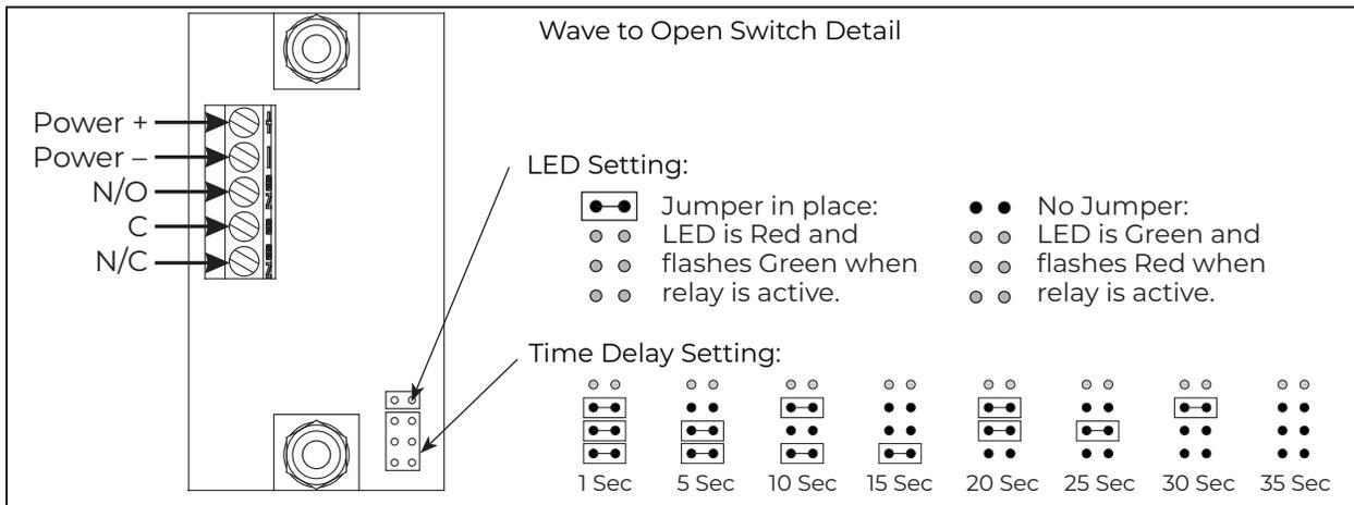
**Standard Activation Wiring Diagram**
