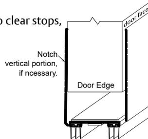
3. Close door and position door bottom shoe so that it makes light even contact with the threshold (ideal overlap is about 1/16"). Mark door in center of slotted holes.
