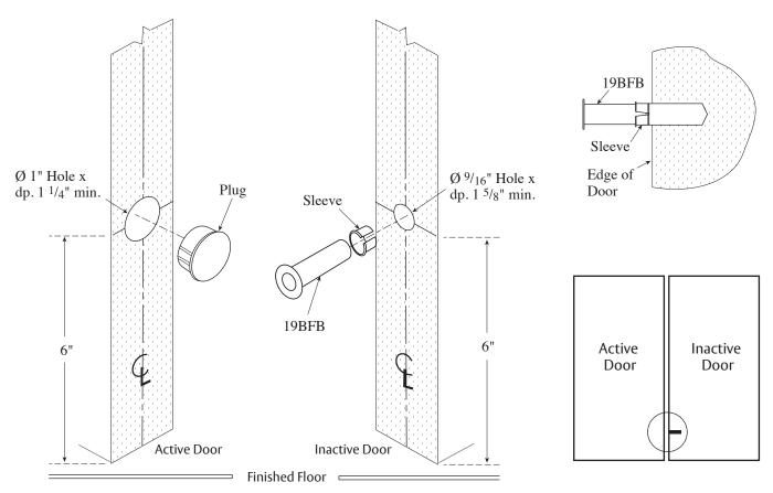
NOTE: Thermal pin to be centered in door thickness; Gap between thermal pin and receiving hole 1/2" max.
