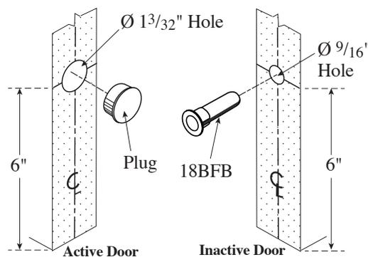
**IMPORTANT:** The 18BFB will project during a fire. Do not cover with any edge mounted door hardware.
