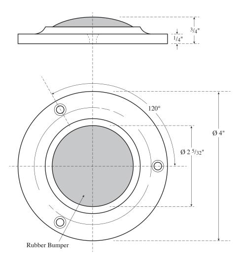
**FASTENERS NOTE:** #8-32 x 2" Round Head Machine Screws and Toggle Bolt
