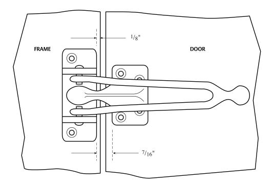
Note: The door guard should be mounted approximately 54" above the floor. (Check with your local authority for any special ADA requirements).
