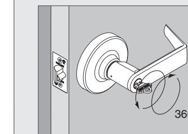
For example, ND66 will lock and unlock with a 360° turn of the key.
