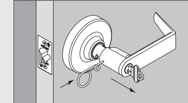
Insert pin wrench and push against lever catch. Pull off the lever.
