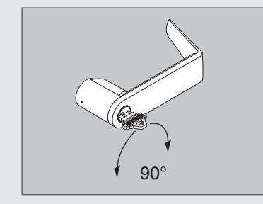
To remove a keyed lever, rotate key 90°.
