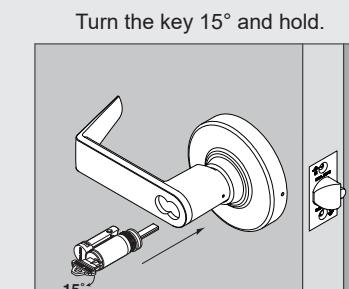
Insert assembly into lever.
