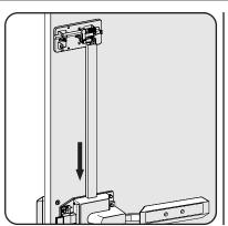
2. The two tabs at the end of channel should rest on the main mechanism mounting plate.
