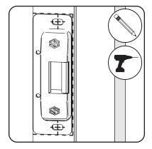
2. Hold the strike plate against the frame with roller facing towards the exterior. Extend bolt and center in strike box. Top of bolt should be approximately 1/8" from top of strike opening.
