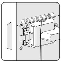
4. Fasten mechanism with (2) 2-1/2" long carriage bolts, (2) K-lock nuts and (2) acorn nuts on hingeside holes. Tighten T-nuts completely.
