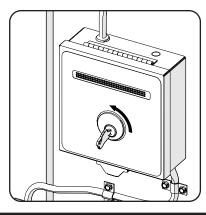
2. If the alarm continues to sound more than 2 times, insert the key and turn clockwise to disarm and see the troubleshooting section. If it stops then the alarm is armed and the key can be removed.
