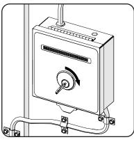
5 Close the lid and screw the anti-tamper screw all the way in. Do not overtighten.
