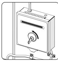
4. Plug battery connectors onto 2 provided 9V batteries and insert into clips as indicated. Be careful to not pull the battery wires when connecting the batteries.
