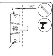
4. Drill 3/4" hole, starting with 1/8" and working up. If needed make the hole egg-shaped toward exterior to prevent bolt from rubbing. Smooth the hole and remove any burrs. Test the bolt operation and make sure that they are not rubbing against hole or binding in any way.
