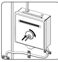
6 Close the lid and screw in the anti-tamper screw located at the bottom of the lid in completely. Do not overtighten. (The alarm will not arm unless this screw is completely inserted).
