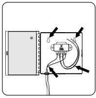
4. Using included cable clips secure the armored cable to the wall as shown.
