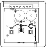
4. Insert a long, slotted head screwdriver into the hole now open where the channel was removed in the main lock and use it to depress the plastic clip as shown.
