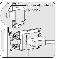
3 Secure (1) 3-1/4" carriage bolt on lock edge opening with (1) K-lock and fasten loosely.
