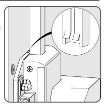
Place cover over module and channel. Make sure tail fits into cover slot.
