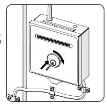
2. Remove the 5mm hex nut from the upper bolt cover on LHR installations or the lower bolt cover on RHR installations and remove the cover.
