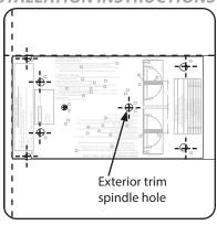
5 Rotate template up vertically and mark top 2 holes. Rotate template down vertically and mark bottom 2 holes.
