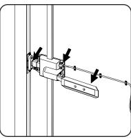
4. If the alarm continues to sound when arming, check to make sure the main deadbolt on the Trident lock is centered in the frame strike. The deadbolt should not rub or lean on the strike roller. Any pressure on the deadbolt will not allow it to extend fully.
