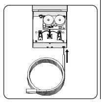
amount of slack in the wires, attach e-clip as shown around the armored cable so it cannot be pulled out.
