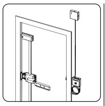
3 Mount the power supply using the hardware appropriate for the installation surface. Mounting screws and anchors are provided.
