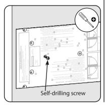
4. Align the top edge of the template with the horizontal line then mark 6 holes on lock edge and exterior trim spindle hole.
