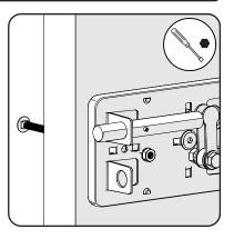
2. To install top bolt module, fasten (1) 2" carriage bolt through the thru-bolt plate with (1) T-nut. Fasten loosely.
