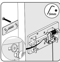
4. Use level to ensure bolt module is level. Tighten T-nut and K-lock nut securely.
