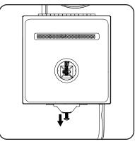
3. Insert the cylinder into the hole in the lid as shown, secure with locking ring.
