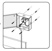
2. Using the indicated holes in the back of the alarm box after positioning, mark the locations to pre-drill holes for mounting hardware.
