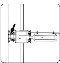
4. Open the lid and remove the two 9 volt batteries from the clips and battery terminals. Be careful to not pull the battery wires when disconnecting the batteries.
