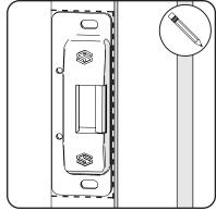
**6.** After final adjustment, secure strike with (2) pan head screws.
