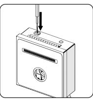
3. Leaving a small amount of slack in the wires, attach e-clip as shown around the armored cable so it cannot be pulled out.
