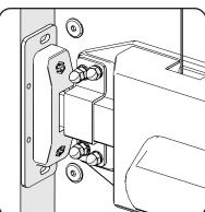
5. Fasten strike to door with (2) self-drilling screws. Test the operation and adjust the position of strike, as necessary.
