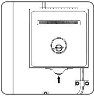
3. Using a Phillips-head screwdriver, unfasten the anti-tamper screw until it spins freely. Do not remove the screw completely.
