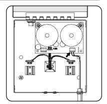
1. Insert the side of the cable with loose wire ends into the rubber grommet on the bottom-right of the alarm box.
