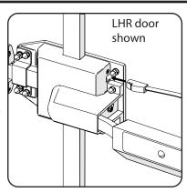
2. Using included cable clips secure the armored cable to the wall, frame, and door as shown. Leave an approximately 10" loop of loose armored cable between the frame and door.
