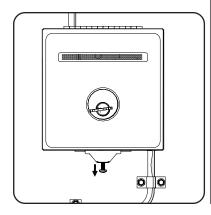
Gently pull the armored cable and wires from the bottom of the box.
