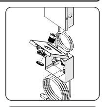
2. Lift the lid and retrieve the cylinder locking ring from inside.
