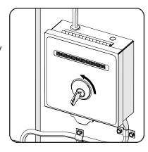
9. If the alarm continues to sound more than 2 times, insert the key and turn clockwise to disarm and see the troubleshooting section. If it stops then the alarm is armed and ready to use and the key can be removed.
