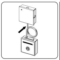
2. Insert stripped wires into the screw terminal indicated and screw down to secure. Polarity does not matter.
