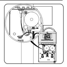
1 Insert the side of the cable with loose wire ends into the rubber grommet on the top-left of the alarm box.
