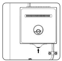
2. Check that the cam on the back of the cylinder depresses the arm and actuates the switch below when turning the key to disarm.
