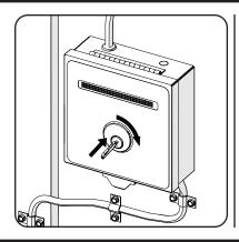
2. If the alarm sounds when disarming, the battery voltage may be critically low. Follow instructions for changing the batteries.
