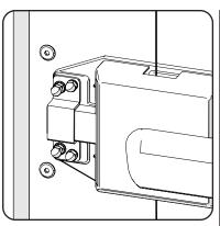
4. Mark centers of oval mounting holes at top and bottom of strike plate. Remove the strike plate. Drill 1/8" diameter pilot holes at center marks.
