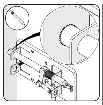
2. Drill 7/8" hole, starting with 1/8" and working up. Smooth the hole and remove any burrs. Test the bolts operation and make sure that they are not rubbing against hole or binding in any way. If needed, grind or enlarge side of the hole that is rubbing against bolt.
