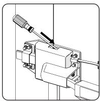
8. Remove cable clips holding the alarm cable to door.
