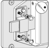
2. Align the top of the mechanism with the horizontal reference line. Use a level to ensure the mechanism is level.
