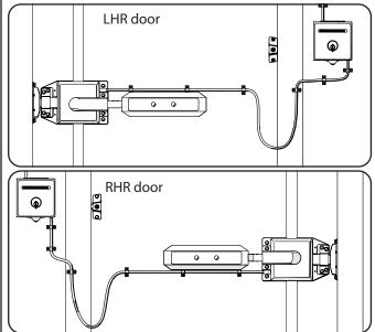
3. Test that the door will open and close without pulling or pinching the armored cable.
