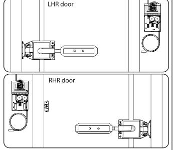
2. Using the indicated holes in the back of the alarm box after positioning, mark the locations to pre-drill holes for mounting hardware.
