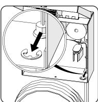
6. Using a Phillips-head screwdriver, unfasten the anti-tamper screw until it spins freely. Do not remove the screw completely.
