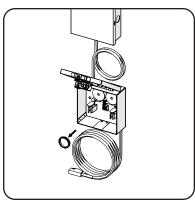
4. Check that the cam on the back of the cylinder depresses the arm and actuates the switch below when turning the key to disarm.
