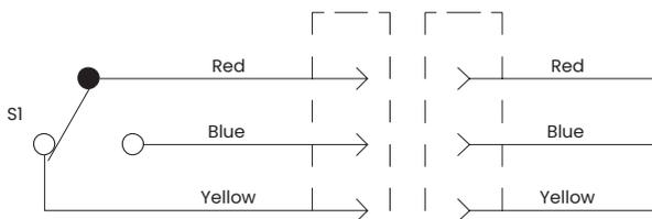
Switch shown with latch status tripper depressed
