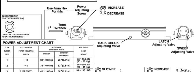
0 (PRESET) 42 "(1.07m) 36 "(0.91m) (45~65 Kg) 143~187 LBS 4 + 3 48 " (1.22m) 42 "(1.07m) (65~85 Kg) 187~264 LBS (85~120 Kg) 5 + 8 54 " (1.37m) 48 "(1.22m) 264~330 LBS 6 + 11 58 " (1.47m) 54 "(1.37m) (120~150 Kg) FASTER SWEEP
