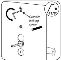
Install cylinder with coil spring and collar into exterior trim by partially inserting key into cylinder and rotating cylinder clockwise into the trim until it bottoms out against the trim back plate. Then rotate counter-clockwise one full rotation to back cam away from back plate.
