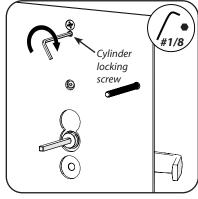
Note: Check operation. If cylinder is rotated too deep into trim, back plate will prevent it from functioning. If this happens, rotate cylinder counterclockwise 1-2 rotations.
