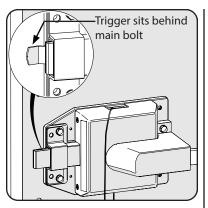
3 Align trim so the spindle fits into hub and posts on plate fit into holes on mechanism.
